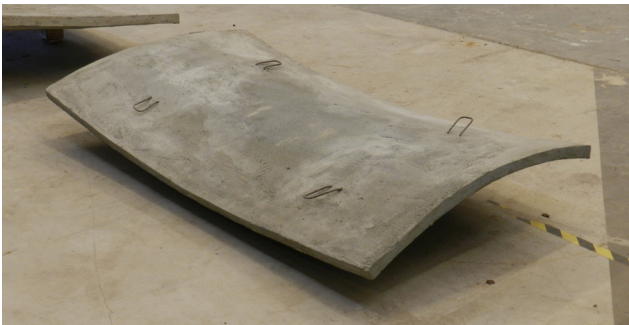
Figure 7: Double-curved panel cast (top) and laser-scanned (below). Source: R. Schipper
